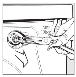
Use water pump pliers to withdraw the plastic filter by the bar (see illustration). Clean, put back and secure.
